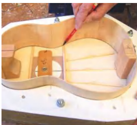
STEP 15. Marking the ends of the harmonic bars
